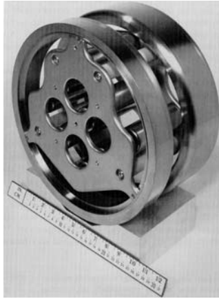
FIGURE 3.3. Geometry of the MBE-4 focusing element.
