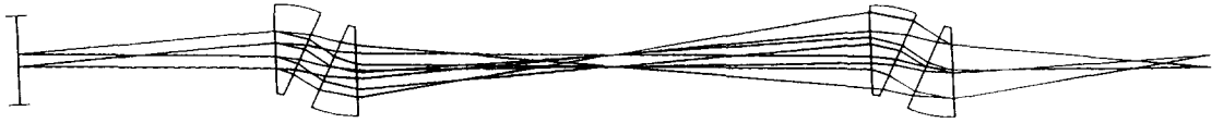
Fig. 2 A simple four cell combined-function magnet achromat without quadrupoles and with a remaining time of flight aberration of about 2 ps.
