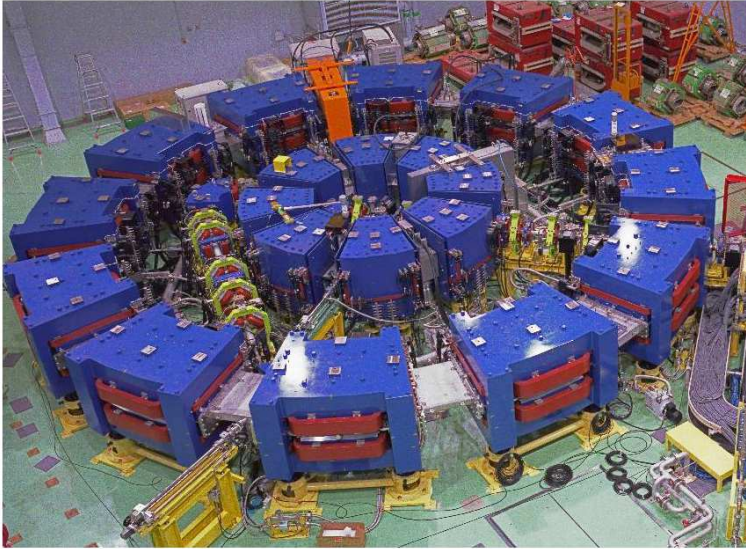
Fig. 11. Cascade of three S-FFAGs for proton acceleration at KURRI. 33
