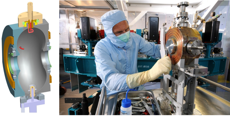
Fig. 4. Design of an EMMA RF cavity (left) and a cavity under test (right).
