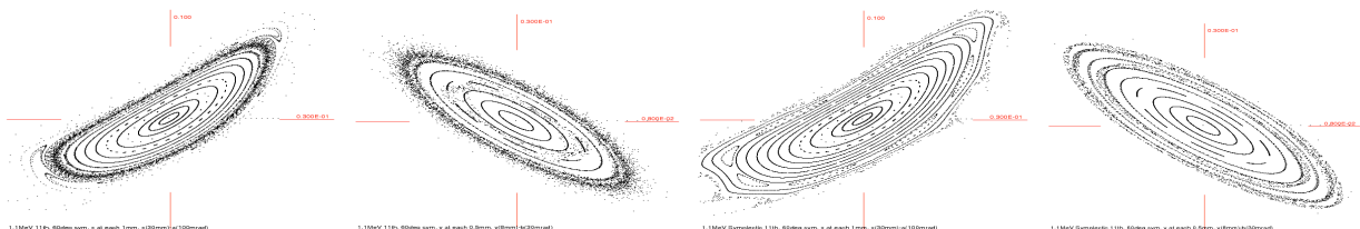
FIGURE 3. Tracking in a model non-scaling FFAG with eleventh-order out of plane expansion, without symplectification (left) and with symplectification (right).
