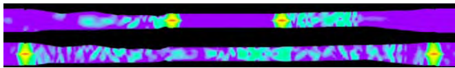
Fig. 15. Beam-excited fields in PEP-II IR from Tau3P simulation before and after two beams passing each other at the collision point.
