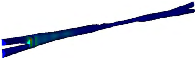
Fig. 16. Omega3P model of the PEP-II IR including placement of absorbers at the crotches.
