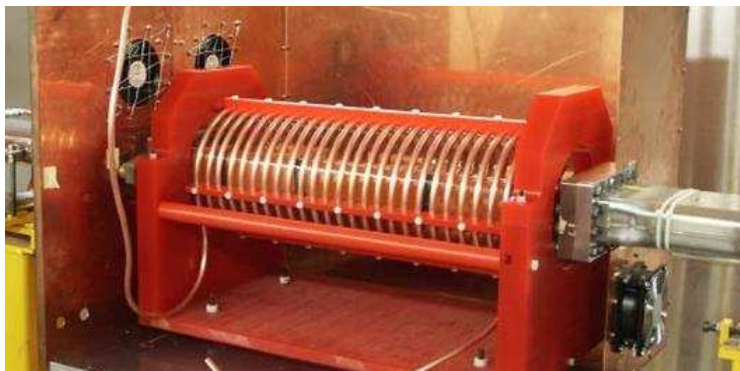
Fig. 7.15: COSY LC-resonant RF solenoid. In COSY, this element precesses the polarization vectors of all particle bunches identically. Its role in the PTR ring will be the same.
