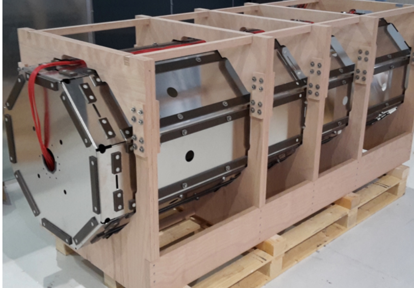
Fig. B.8: Magnetic shielding prototype, developed in collaboration with Fierlinger Magnetics, Germany. It contains two layers, 1 mm thick, of high-permeability material, separated by \approx 10 cm and is approximately 2.5 m long.
