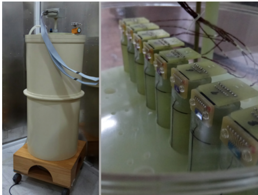
Fig. B.5: Time-averaging measurements were made with a set-up having the same electronics but different designs of the (left) dewar and (right) gradiometer [2]. The figure is licensed under CC-BY-4.0 .
