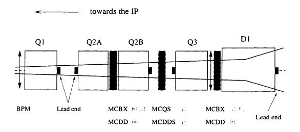
Figure 4.3: Layout of the left low- $\beta$  triplet.
