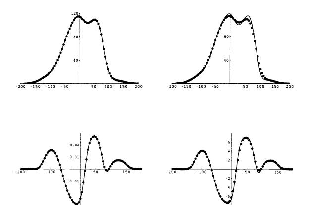
Figure 5.7: Comparison of the skew multipoles  $a_{2,2}$  (top) and  $a_{6,6}$  (bottom) with  $\overline{a}_2$  respectively  $\overline{a}_6$  in the lead end for r = 5 mm (left) and r = 20 mm (right).
