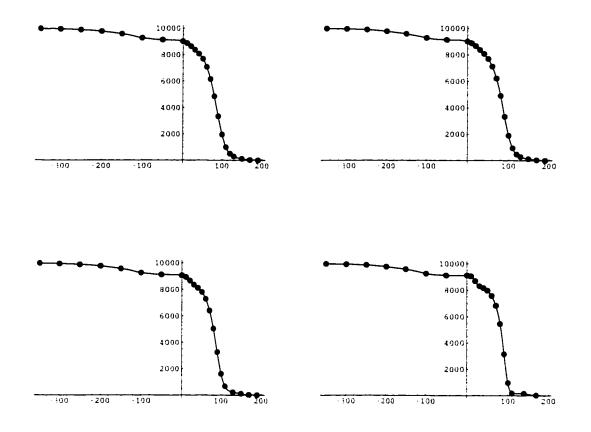
Figure 5.4: Comparison of  $\bar{b}_2$  in the lead end as computed by the differential algebraic field calculation in COSY and as given in [23] for different radii. From top left to bottom right : r = 5 mm, r = 10 mm, r = 20 mm and r = 30 mm.
