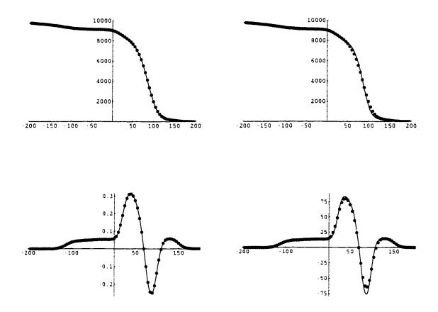
Figure 5.6: Comparison of the normal multipoles  $b_{2,2}$  (top) and  $b_{6,6}$  (bottom) with  $\bar{b}_2$  respectively  $\bar{b}_6$  in the lead end for r = 5 mm (left) and r = 20 mm (right).
