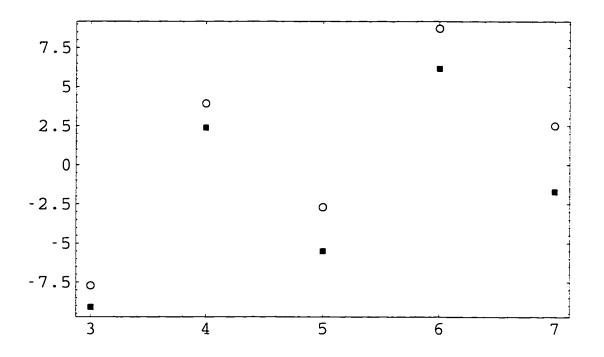
Figure 4.5: Average logarithmic resonance strength for orders 3 to 7. The values are given by squares for the case without fringe fields and circles for the case with fringe fields.
