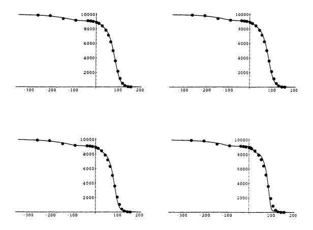
Figure 4.2: Comparison of the quadrupole component of the field in the lead end as computed by COSY and ROXIE at different radii. From top left to bottom right: r = 5 mm, r = 10 mm, r = 20 mm and r = 30 mm.
