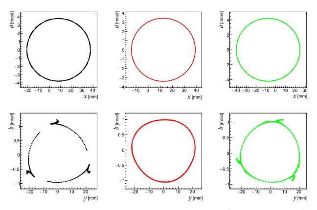
Figure 3.40: Trajectories in phase space of three different muons (distinguished by color) in the nonlinear regime.
