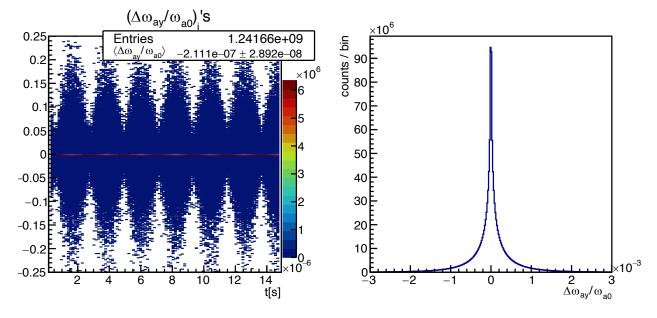
Figure 4.21:  $\langle \Delta \omega_a \rangle$  spread distribution (right) and versus time (left). Muons are launched with no radial motion nor momentum offsets, to exclude  $C_e$ . The frequencies spread due to the  $C_p$  correction is 0.1% as shown in the plot on the right.
