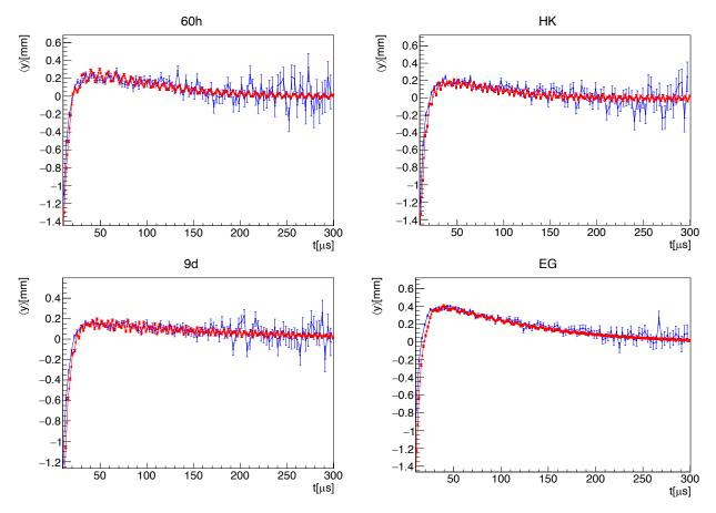
Figure 3.81: Vertical centroid from simulated beam (red) and tracker data (blue), station 12 for each Run-1 dataset.
