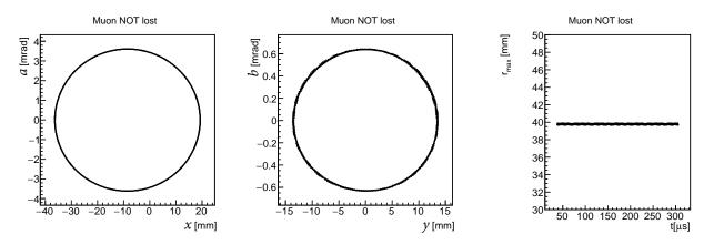
Figure 3.36: Phase space coordinates and maximum excursion of a muon not lost (reference case).
