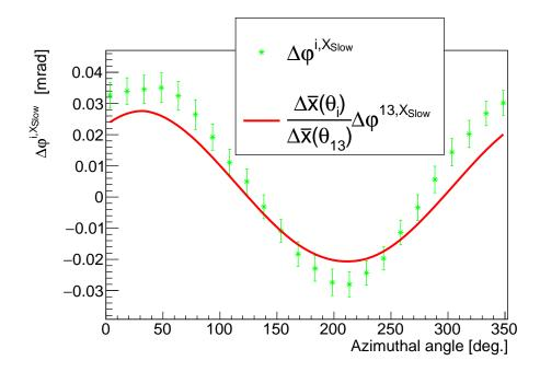
Figure 4.13: Drifting phase amplitudes from single-exponential fits to phase drifts (extracted from non-randomized, sliding window fits) induced by radial slow beam drifts. In red, scaling of the phase amplitude at calorimeter k = 3 with radial beam centroid drifts only.
