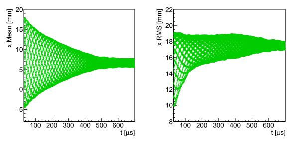
Figure 3.47: Long-term radial beam de-coherence.
