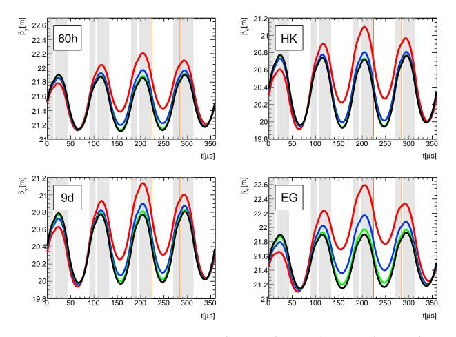
Figure 3.69: Vertical beta functions at 30  $\mu$ s (red curves), 100  $\mu$ s (blue curves), 200  $\mu$ s (green curves), and 300  $\mu$ s (black curves) during Run-1.
