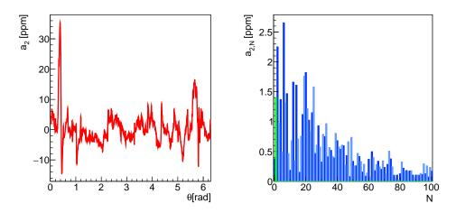
Figure 3.34: On the left, magnetic skew sextupole coefficient  $a_2$  as measured by NMR probes. On the right plot, Fourier decomposition of the coefficient  $a_2$  in azimuthal harmonics  $a_2 = \sum_{N=0}^{n} a_{2,N} \cos (N\theta + \phi_N)$ . The N = 1 term, which is the main driver of the resonant condition  $3\nu_y = 1$ , is depicted in green color.
