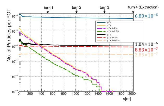
Figure 2.5: Number of muons,  $\mu^+$ , pions,  $\pi^+$ , and protons,  $p^+$ , per proton on target (POT) along four turns around the Delivery Ring. The design momentum acceptance of 2% reveals naturally in beam tracking simulations when accounting for the beamline apertures present in the DR. All pions decay prior to the third turn along the DR.
