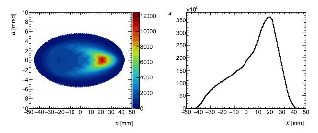
Figure 3.54: Radial phase space at late times of the data taking period (left) and its spatial projection (right) from Run-1 simulation. The pattern closely resembles observations and its characteristic skewness is present in all Run-1 datasets.
