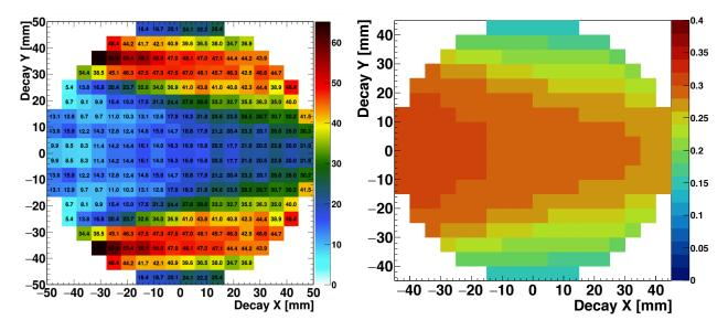
Figure 4.7: Typical detected-phase  $\varphi_{0,k}$  (left) and calorimeter acceptance  $\varepsilon_{c,k}$  (right) maps from GM2RINGSIM [44]. In the phase map, values indicated by the color legend (in mrad) are relative to a central g-2 phase defined at injection. 1 µrad phase shifts over a muon lifetime in the laboratory frame induce  $\omega_a$  shifts of about 10 ppb.
