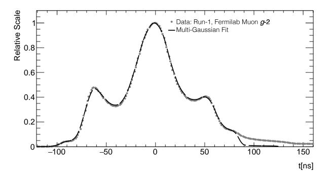
Figure 3.14: Representative longitudinal profile of the muon beam as measured by the T0 detector. Its length is desired to be contained within the main peak of the kicker pulse to maximize beam storage. The solid line shows the type of multi-Gaussian interpolation used in the model to recreate the longitudinal profile of the simulated muon beam.
