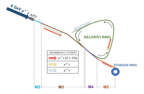
Figure 2.1: A schematic layout of the beam delivery system (BDS). Secondary particles (mostly pions, muons, and protons) downstream of the target station at AP0 are canalized through the M2/M3 lines and injected into the Delivery Ring (DR), where protons are discarded and most of the remaining pions decay after four turns. A cleaner beam of mostly muons is extracted to the M4/M5 lines and ultimately delivered to the Muon g-2 Storage Ring (SR).
