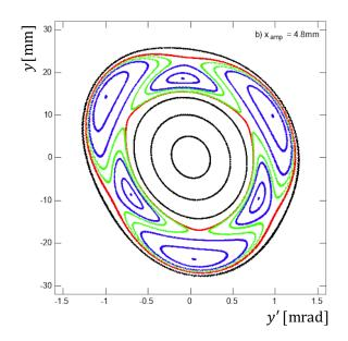
Figure 3.44: Stroboscopic tracking in the vertical phase space illustrating orbit behavior with two period-3 fixed point structures present [101], for ESQ voltage at 18.3 kV. Trajectories in blue and green colors are examples of muons (within the ring admittance and momentum acceptance) with highly modulated vertical amplitudes. Picture by courtesy of Adrian Weisskopf.
