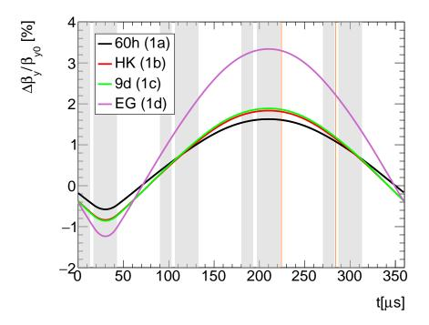
Figure 3.72: Relative vertical beta functions drift from  $30 \,\mu s$  to  $1000 \,\mu s$ .
