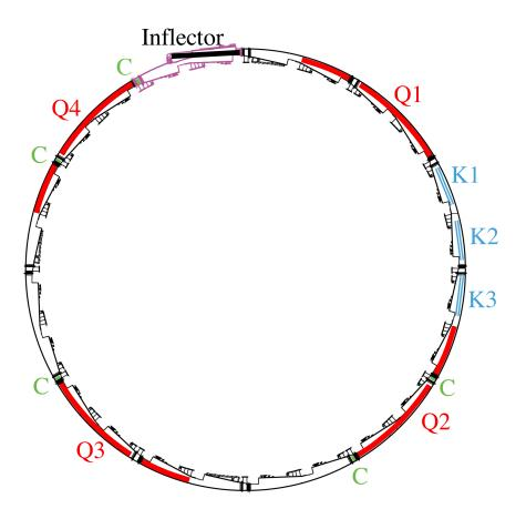
Figure 3.1: Layout of the Muon g-2 storage ring at Fermilab. The four locations of the ESQ are found next to labels "Q1-Q4" (each covering 39° azimuthally) and labels "K1-K3" indicate the place of the injection kicker plates within the ring. "C" labels denote the beam collimators arrangement.
