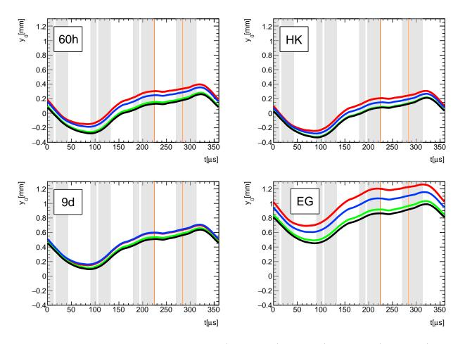
Figure 3.68: Vertical closed orbits at 30  $\mu$ s (red curves), 100  $\mu$ s (blue curves), 200  $\mu$ s (green curves), and 300  $\mu$ s (black curves) during Run-1. Gray shadows depict ESQ stations along the azimuth, where the Q1S upstream edge is at  $\theta = 0$ . Orange lines indicate collimator locations. Red curves are subject to the effects of the ESQ scraping configuration and the green curves have almost reached the equilibrium values.
