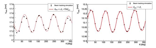
Figure 3.57: Comparison between beam widths from optical lattice functions (red curves) and randomized beam widths from Run-1 tracking simulations.
