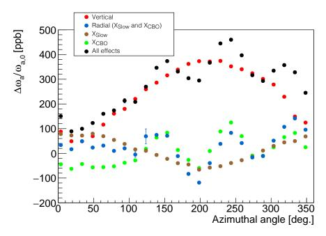
Figure 4.16: Relative  $\omega_a$  shifts induced by each of the drifting phase mechanisms, separated and combined. The largest shifts are produced by beam drifts of the vertical width.
