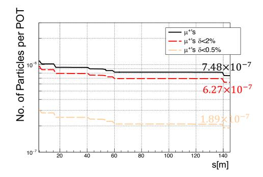
Figure 2.8: Number of muons,  $\mu^+$ , per proton on target (POT) along the M4/M5 beamlines. The pale-rose dashed line depicts muons within the muon g-2 storage ring momentum acceptance. For g-2 runs posterior to Run-1, the insertion of passive wedge absorbers in the BDS maximized the muon population within  $|\delta| < 0.5\%$  to increase the stored beam fraction [62].
