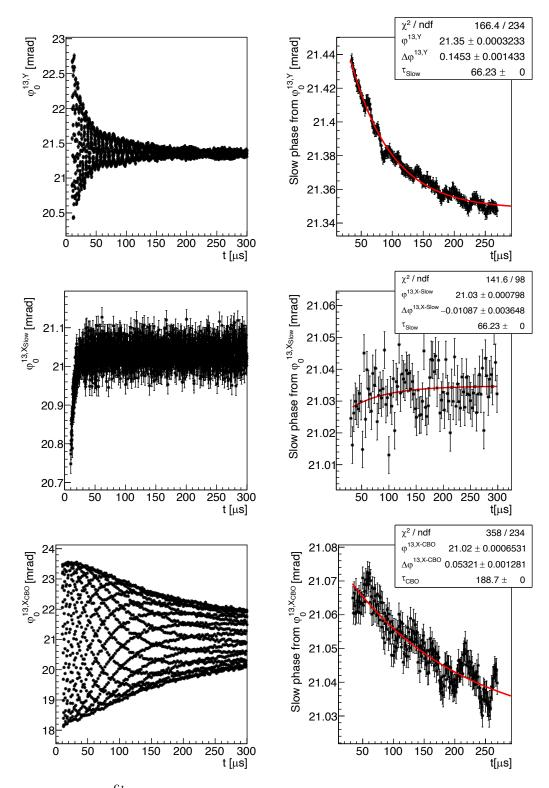
Figure 4.11: Phases  $\varphi_0^{c_k}(t)$  (left) and their corresponding phase drifts (on the right) from the non-randomized, window fits method. The two plots on top correspond to a detected phase at calorimeter k = 13 from vertical beam drifting. In the middle, phase changes are driven by slow radial beam motion. At the bottom, phase drifting due to radial CBO de-coherence. Fits in red are performed to extract drift amplitudes.
