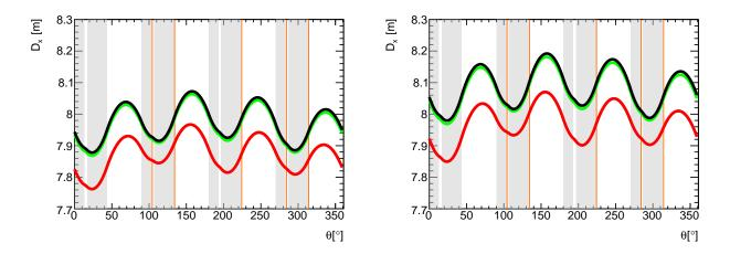
Figure 3.19: Radial dispersion function at 5  $\mu$ s (red curves), 20  $\mu$ s (green curves), and 1000  $\mu$ s (black curves). The ESQ voltage is equal to HV = 18.3 kV on the left-side plot, whereas HV = 20.4 kV for the plot on the right side. Inhomogeneities in the normal quadrupole term of the magnetic field break the four-fold symmetry.
