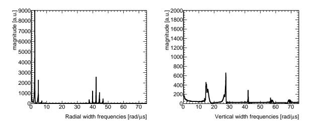
Figure 3.50: Beam frequencies extracted with FFT from widths motion.
