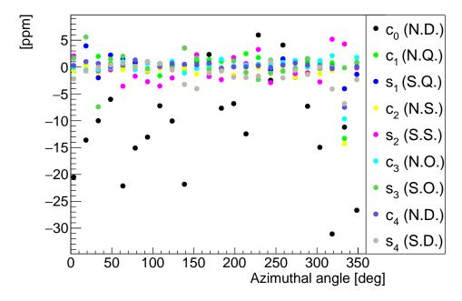
Figure 4.30: Magnetic field multipoles averaged out every  $15^{\circ}$  (trolley run 3956). Refer to Eq. (4.37).
