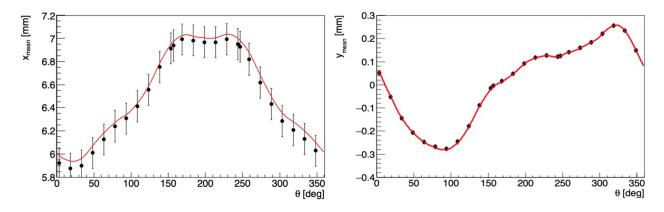
Figure 3.56: Comparison between closed orbits (red curves) and randomized beam centroids from Run-1 tracking simulations.
