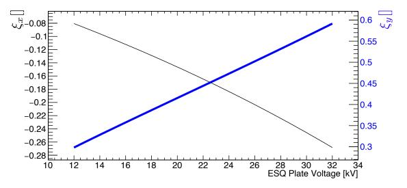
Figure 3.16: Radial (black) and vertical (blue) linear chromaticities as a function of ESQ voltage.
