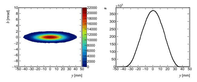
Figure 3.55: Vertical phase space at late times of the data taking period (left) and its spatial projection (right) from Run-1 simulation.
