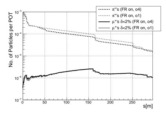
Figure 2.11: Simulation results of the number of pions and muons with  $|\delta| < 2\%$  per POT under up to fourth-order (o4) effects along the M2/M3 lines with fringe fields (FR) turned on. The longitudinal distance along the M2/M3 lines is shown in the horizontal axis. As depicted by the overlapping curves of the muon population for the two o1/o4 cases, linear simulations do not significantly differ from results when high-order terms in the computation of the particle dynamics are simulated.
