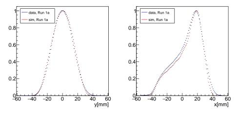
Figure 3.78: Muon beam intensity projections from simulation (red) and tracker data (blue), station 12, during Run-1a from  $30 \,\mu s < t < 300 \,\mu s$ .
