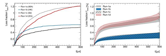
Figure 4.3: Muon loss rates versus time, 30 µs after injection, from symplectic tracking Run-1 simulations (left) and data (right, [119]). The  $3\nu_y = 1$  resonance nearby Runs 1a and 1d increases the loss fraction (Sec. 3.4.3). Uncertainty bands on the curves from data accounts for experimental scaling errors in the determination of muon loss rates.
