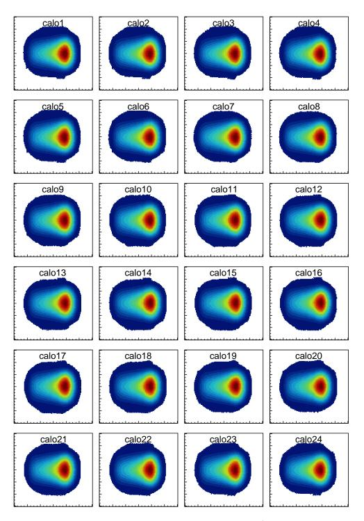
Figure 4.26: Run-1a simulated beam transverse profiles  $M_T^{orig}(x_j, y_k, \theta_i)$ , integrated over  $30 \,\mu\text{s} < t < 300 \,\mu\text{s}$ . The 24 azimuthal locations coincide with the regions of maximum calorimeter detection acceptance. Horizontal and vertical axes correspond to  $-60 \,\text{mm} < x < 60 \,\text{mm}$  and  $-60 \,\text{mm} < y < 60 \,\text{mm}$ . Refer to Fig. 4.36 for the color legend.
