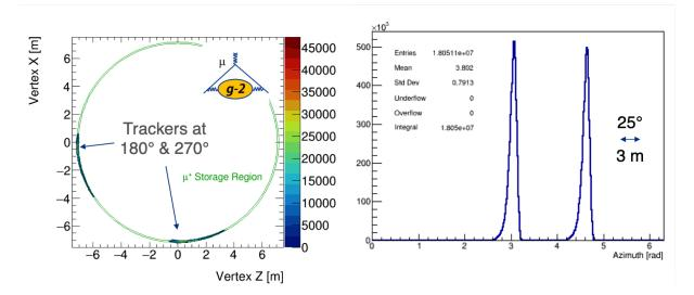
Figure 1.11: Horizontal (left) and longitudinal (right) acceptances of the two g-2 straw tracker detector stations [43]. Each tracker station reads decay vertexes along azimuthal segments of  $\approx 0.4$  mrad, whose maximum acceptance peaks are positioned at about 1 m upstream of the modules.
