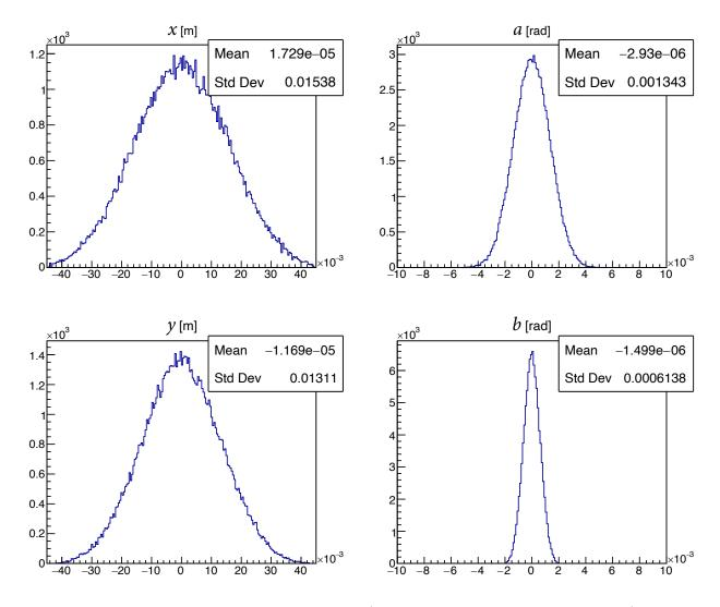
Figure 4.18: x - a - y - b beam distributions (matched to the ring optical lattice) used in tracking simulations for  $C_{e,p}$  analysis.
