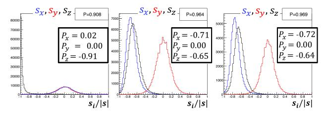
Figure 2.10: Histograms of the normalized muon beam spin components (in natural units) in optical coordinates at the end of M3 (left), Delivery Ring (center), and M5 (right) beamline sections. The polarization projections  $P_x$ ,  $P_y$ , and  $P_z$  (parallel to the x, y, and s directions, respectively) are shown inside the thick black frames. As indicated by the projection  $P_y = 0$ , the high polarization P of the beam is largely contained in the horizontal plane.
