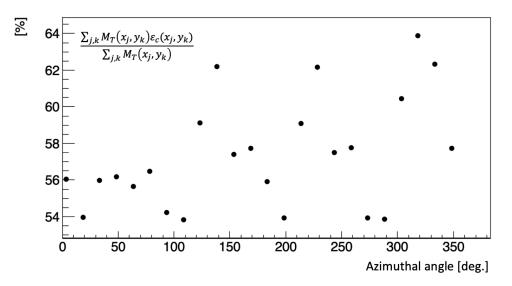
Figure 4.15: Convolution of total intensities detected by each calorimeter (T-Method) using the COSY-based Run-1a simulated beam and GM2RINGSIM acceptance maps. The formula on the top-left corner indicates the weighting of the beam intensity with muon detection efficiency.
