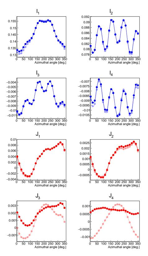
Figure 4.40: Multipole beam projections  $\{I_{n,i}, J_{n,i}\}$  versus azimuthal angle from the Run-1a simulated beam (semi-transparent colors) and reconstructed profiles (solid colors). The small contributions from the skew octupole and decapole projections are not well transformed in the reconstruction.
