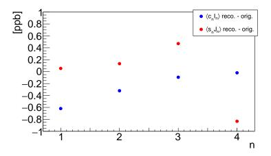
Figure 4.39: Comparison of weighted field contributions from each magnetic multipole moment using beam projections from the reconstructed versus the original muon distribution.
