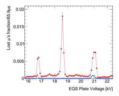
Figure 3.35: Lost muons fraction over a muon lifetime after the scraping stage is completed. In red (triangular markers), all the magnetic multipole terms are turned on during the beam tracking simulation, whereas in blue (diamond markers), these are turned off. In subsequent simulations, it was found that only the magnetic skew sextupole term from measured field inhomogeneities was sufficient to drive the betatron-resonance peak at  $HV \approx 18.6$  kV.
