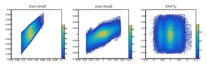
Figure 3.13: Simulated beam distribution at the exit of the inflector, after the final focus to pass the beam through the hole in the backleg iron. The beam is mostly tangential to the design orbit and about 77 mm radially outward at injection.
