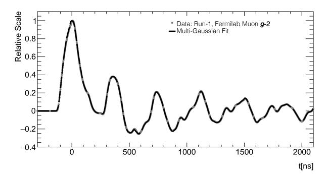
Figure 3.10: Representative kicker strength pulse during the first run of the muon g-2 experiment, measured with a magnetometer.
