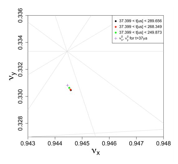
Figure 3.39: Tunes of three lost muons in the linear regime. Note the proximity between the red and black entries (the red marker partially covers the marker in black color).
