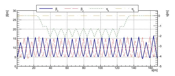
Figure 2.6: Beta and dispersion functions at one three-fold symmetric section of the delivery ring (DR) where the longitudinal distance of the beamline is shown in the horizontal axis. Fringe fields modeled in simulations change the beta functions,  $\beta_x$  and  $\beta_y$ , by less than 3%.
