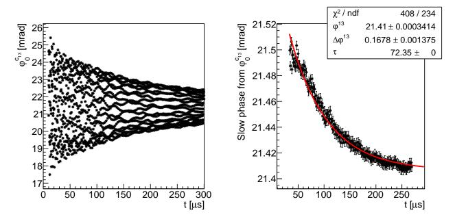
Figure 4.8: On the left side, the phase  $\varphi_0^{c_{13}}(t)$  from the COSY-based Run-1a simulated beam and GM2RINGSIM maps (T-Method) via Eq. (4.12). On the right, the phase drift extracted from non-randomized window fits (black markers), which effectively capture the phase drift without the modulation induced by the beam coherent oscillations shown on the left plot. The red curve is a single-exponential fit to the resulting phase drift without modulation.
