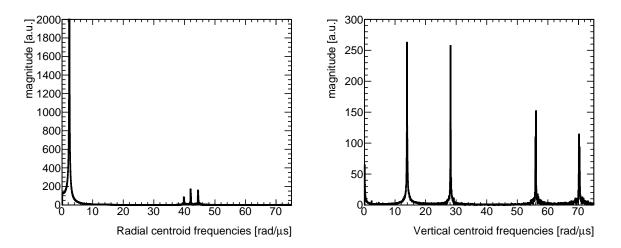
Figure 3.49: Beam frequencies extracted with FFT from centroids motion.
