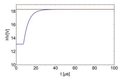
Figure 3.4: Illustration of the HV traces from plates connected to the 1-pulse (red line) and 2-pulse (blue curve) HV supplies. The mis-powered ESQ plates (blue) during the initial  $\sim 7 \,\mu s$  after injection shift the beam towards the limiting apertures of the storage volume, in order to scrape the beam in preparation for the data taking period at  $t > 30 \,\mu s$ .
