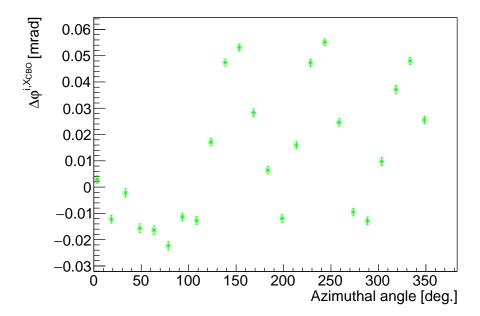
Figure 4.14: Drifting phase amplitudes from single-exponential fits to phase drifts (extracted from non-randomized, sliding window fits) induced by radial CBO de-coherence. Variations are largely caused by calorimeter acceptances, which exhibit a characteristic azimuthal pattern owing to the instrumentation between the storage volume and the calorimeter detectors (see Fig. 4.15).
