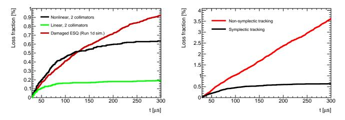
Figure 3.45: Muon loss rates from several tracking simulations (HV=18.3 kV). The effect of damaged resistors and the effect from symplectic enforcement during tracking is shown.
