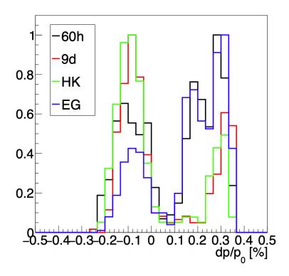
Figure 4.4: Relative momentum offsets of lost muons from Run-1 symplectic tracking simulations ( $30 \ \mu s < t < 300 \ \mu s$ ). The vertical axis indicates the number of lost muons (in arbitrary units) per bin of momentum offset.
