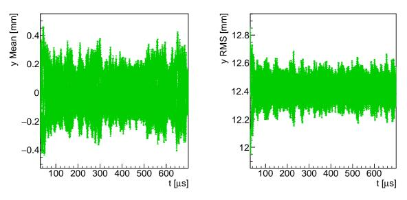
Figure 3.48: Long-term vertical beam temporal modulations.
