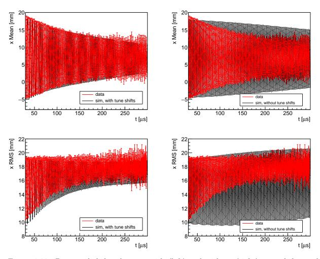
Figure 3.29: Beam radial de-coherence with (left) and without (right) tune shifts at the readout location of the straw tracking detector (station 12). As a reference, data from the tracker is shown in red. The two plots on top display radial beam centroids, whereas the bottom plots correspond to radial beam widths.
