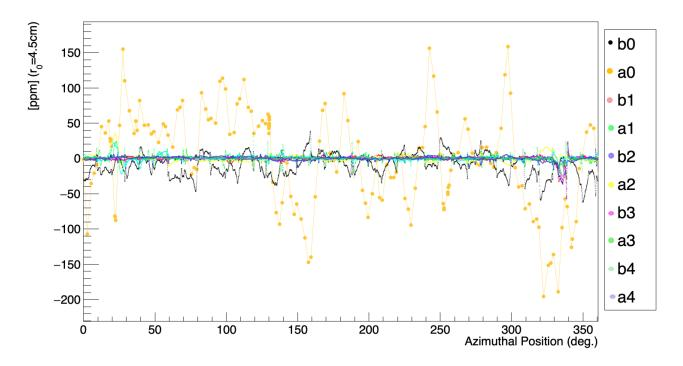
Figure 3.8: Magnetic field multipoles from Trolley Run 3956. All the multipole terms are expressed relative to the ideal vertical magnetic field  $B_0$  that sustains magic muons in the ideal orbit. The skew dipole term (also called radial field) was measured with a Hall probe in 2016 [40] and averaged out to recreate the expected effect of the surface correction coils (SCC).
