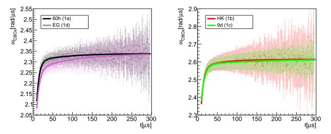
Figure 3.60: Radial CBO frequencies during the four Run-1 datasets from straw tracking detectors data. Semi-transparent markers are obtained from sliding sinusoidal fits ( $\pm 5 \,\mu s$ ) to the recorded radial beam centroid, whereas solid lines result from multi-parameter fits through the entire fill. Both methods are equivalent.
