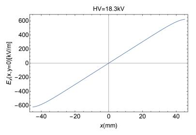
Figure 3.5: Radial electric field along the midplane (HV= 18.3 kV). Near the aperture limits at x = 45 mm, nonlinearities from the ESQ electric fields distort the otherwise linear radial field.
