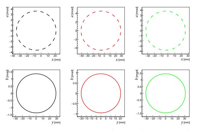
Figure 3.37: Trajectories in phase space of three different muons (distinguished by color) in the linear regime.
