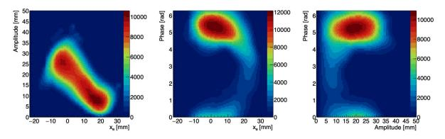
Figure 3.76: Reconstructed beam distribution in the radial direction. On the left plot, the upper limits are determined by the physical apertures of the collimators which bound maximum radial excursions, whereas the maximum kicker strength defines the lower limits.
