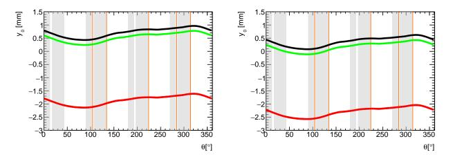
Figure 3.24: Vertical closed orbits ( $\delta = 0$ ) at 5 µs (red curves), 20 µs (green curves), and 1000 µs (black curves). On the left-side plot HV = 18.3 kV, whereas HV = 20.4 kV for the plot on the right side. The induced skew dipole ESQ field created from the HV imbalance between the top/bottom plates shifts the vertical closed orbit for beam scraping.
