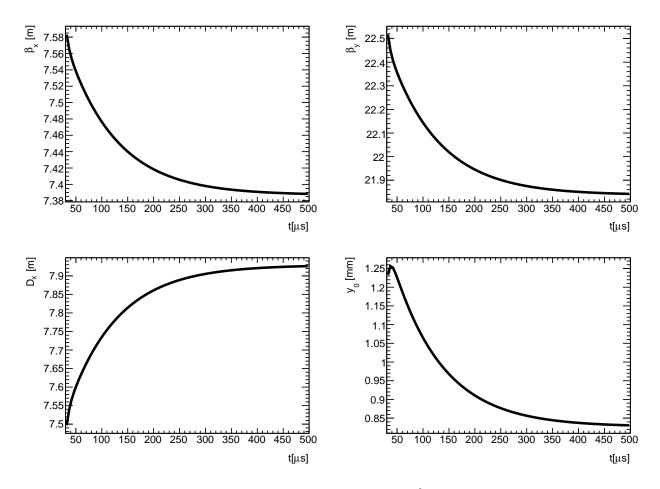
Figure 3.73:  $\beta_x$ ,  $\beta_y$ ,  $D_x$ , and vertical closed orbit at 210° from the upstream entrance of station Q1S for dataset Run-1d.
