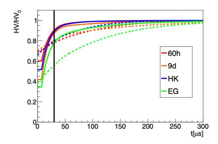
Figure 3.65: Reconstructed HV traces (normalized to their nominal voltage set-points) at Q1L during Run-1 datasets. Dashed and solid lines correspond to Q1LT and Q1LB plates, respectively.
