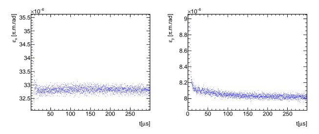
Figure 3.53: Beam emittances from tracking. Due to the smaller vertical admittance, the vertical emittance is more affected by muon loss rates.
