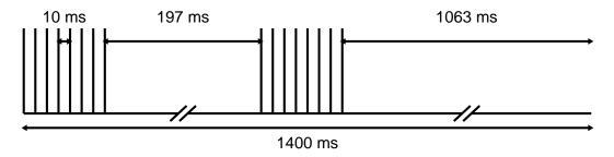
Figure 2.2: Time structure of the  $10^{12}$ -, 120 ns-pulse train impinging the production target per cycle [55].
