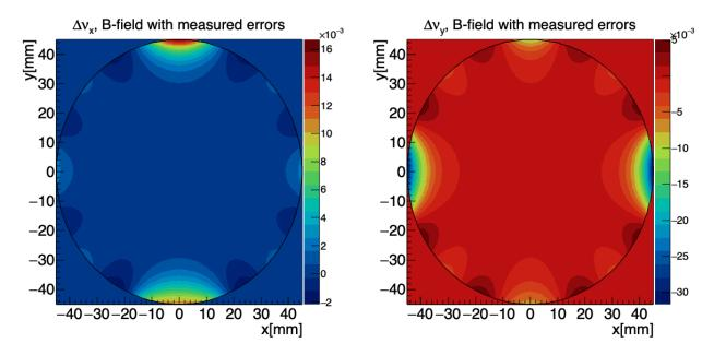
Figure 3.27: Amplitude-dependent tune shifts ( $\delta = 0$ ) within the storage region with magnetic field imperfections (HV= 18.3 kV). The horizontal axis corresponds to radial betatron amplitudes and the vertical axis represents vertical amplitudes.
