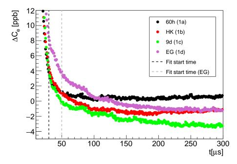
Figure 4.25: Temporal  $C_e(t)$  corrections (relative to the time-independent case) during Run-1 under the effects of changing momentum spread and time-dependent ESQ electric fields.
