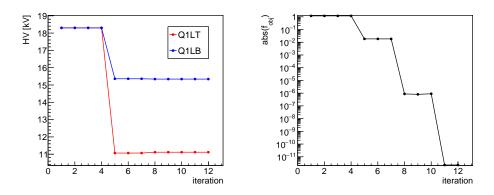
Figure 3.64: High voltage on Q1LT and Q1LB plates (left) and objective function (right) per iteration as the optimization takes place for the Run-1, EndGame dataset, at 40  $\mu$ s. The optimizer supported by COSY INFINITY (i.e., the generalized least squares Newton method) fits Q1LT/Q1LB HVs such that the COSY-based storage ring model with damaged resistors accounted for reproduces a vertical fixed point (equivalent to the vertical mean) and CBO frequency as measured by tracker station 12.
