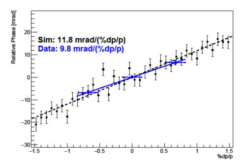
Figure 4.1: Momentum dependence of the initial g-2 phase  $\varphi_0$ . The simulations (black plot markers) are in good agreement with experimental data (blue, preliminary). The experimental data were obtained by studying the behavior of muons with momenta above and below the magic momentum in the storage ring [118].
