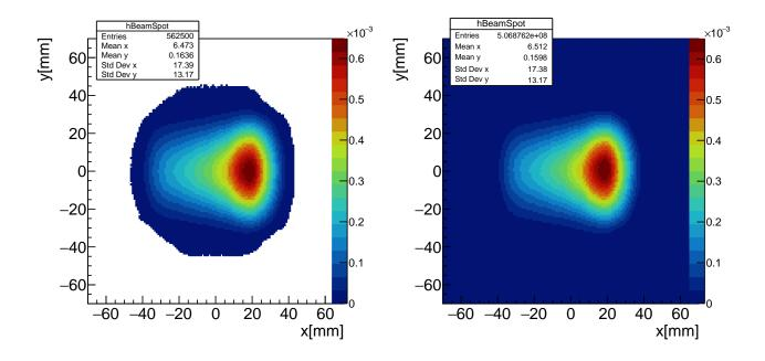
Figure 4.36: Reconstructed  $M_T^{reco}(x, y)$  (left) and original  $M_T^{orig}(x, y)$  (right) beam transverse profiles azimuthally averaged and integrated in time (30 µs < t < 300 µs).
