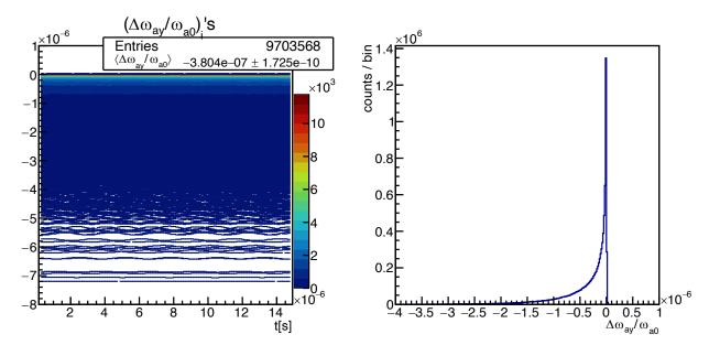
Figure 4.20:  $\langle \Delta \omega_a \rangle$  spread distribution (right) and versus time (left). Muons are contained within the horizontal midplane to exclude  $C_p$ . Typical frequency spreads due to the  $C_e$ correction are approximately equal to ~ 540 ppb, as observed from the standard deviation in the right plot.
