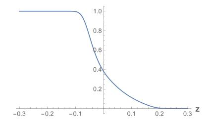
Figure 2.12: Enge function falloff of a typical dipole element in COSY INFINITY, used to represent fringe fields in the BDS simulations. The aperture for this case is equal to 10 cm.
