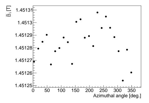
Figure 4.28:  $\tilde{B}_i$  magnetic fields (trolley run 3956) weighted with the Run-1a simulated beam at 24 azimuthal locations.
