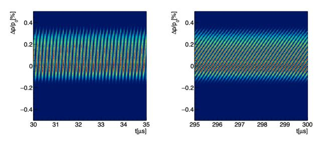
Figure 4.2: Momentum spread over time from Run-1d tracking simulations at early and late times. While the beam spreads in the longitudinal direction, muons with different momenta combine together.
