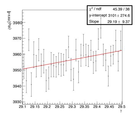
Figure 2.16: Beam average of the spin projection angle in the horizontal plane with respect to the reference optical axis,  $\langle \varphi_a \rangle$ , versus the Lorentz factor,  $\gamma$ , at the exit of the delivery ring after four turns. Simulation results presented in this figure correspond to our COSY-based BDS model with fringe fields turned on.
