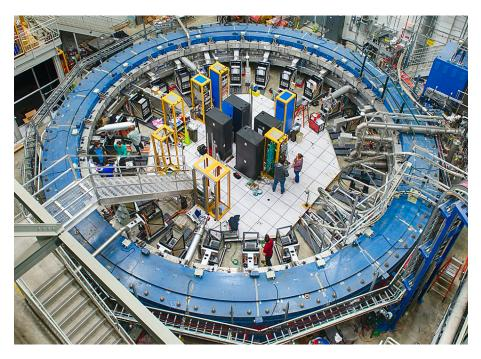
Figure 1.8: Muon g-2 storage ring housed at Fermilab. The steel yokes and superconductive coils crossed thousands of miles from Brookhaven National Laboratory to Fermilab for extended use. After the first data-taking period at Fermilab, the storage ring magnet was covered with thermal insulation to reduce temperature gradients that affect the uniformity of the magnetic field.
