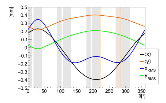
Figure 3.74: Beam drifts from 40  $\mu$ s to 300  $\mu$ s anchored to tracker data for the Run-1d dataset. Gray shadows depict ESQ stations along the azimuth, where the Q1S upstream edge is at  $\theta = 0$ . Orange lines indicate collimator locations. With the Run-1 optical lattice functions, the observed beam drifts measured by the muon g-2 straw tracking detectors are projected along the entire azimuth of the storage ring.
