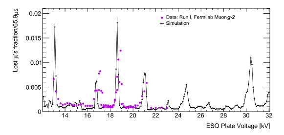
Figure 3.30: Fraction of muon losses between  $121 - 186 \,\mu s$  after beam injection with the COSY-based model for several ESQ configurations. Measurements [94]—shown in arbitrary units—result from detections of minimum ionizing particles that deposit ~ 170 MeV of energy in two adjacent calorimeters while two collimators were inserted to the storage region.
