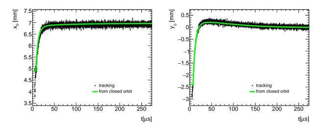
Figure 3.51: Comparison between closed orbit and beam centroid from tracking at  $157^{\circ}$  downstream from the entrance of Q1S. Tracking data is randomized to remove beam beating from mismatch. The initial distribution and guide fields are prepared for the 60*h* case as explained in Sec. 3.6.
