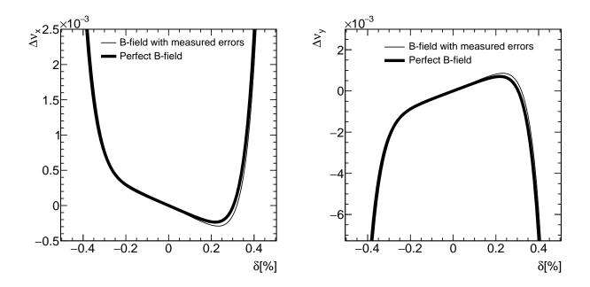
Figure 3.28: Momentum-dependent tune shifts (no betatron amplitudes) with and without magnetic field imperfections (HV= 18.3 kV). Nonlinear shifts take place for  $|\delta| > 0.2\%$ , inside the momentum acceptance.
