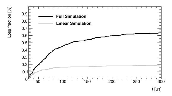
Figure 3.43: Muon loss fractions with nonlinearities (black curve) and without them (gray curve) from symplectic tracking, COSY-based, beam simulations. The ESQ setpoint was 18.3 kV, two collimators were inserted, and both cases start with the same data-based initial distribution. Muon loss rates are highly affected by nonlinearities of the guide fields.
