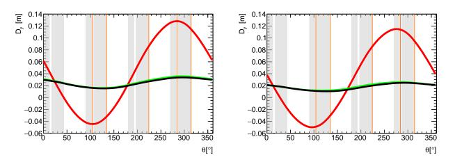
Figure 3.20: Vertical dispersion function at  $5 \,\mu s$  (red curves),  $20 \,\mu s$  (green curves), and  $1000 \,\mu s$  (black curves). On the left-side plot HV =  $18.3 \,\mathrm{kV}$ , whereas HV =  $20.4 \,\mathrm{kV}$  for the plot on the right side. As the magnetic field is mostly oriented vertically, vertical dispersions are negligible.
