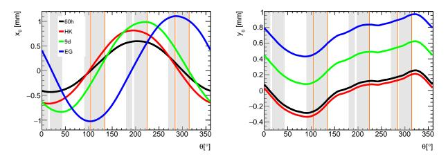
Figure 3.25: Representative closed orbits during the datasets of the first run (Run-1) of the experiment (60h (1a), HK (1b), 9d (1c), and EG (1d)). Fluctuations in temperature affected the dipole terms of the magnetic field, which led to different closed orbits per Run-1 dataset.
