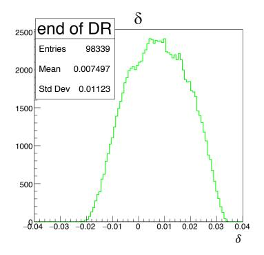
Figure 2.9: Momentum spread of the muon beam after four turns around the Delivery Ring. The momentum acceptance sustained at the BDS beamlines allows for the preparation of a highly polarized muon beam (P=0.969 from BDS simulations).
