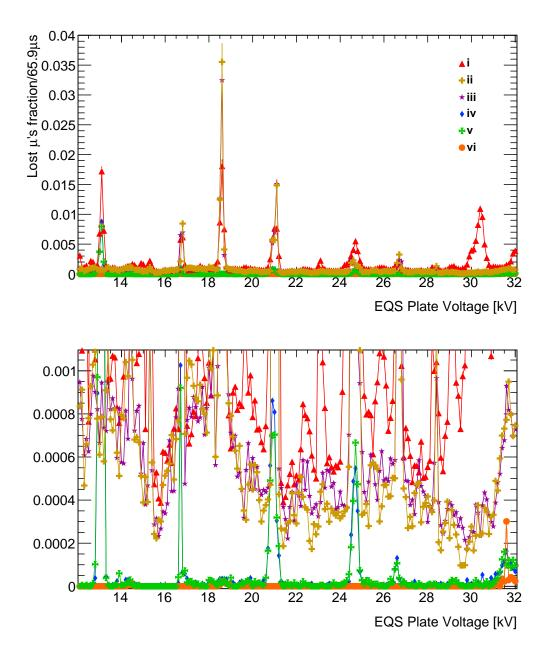
Figure 3.33: Fraction of muon losses from simulations during the time interval  $121 - 186\mu$ s after beam injection. Configuration details are listed on page 116. The bottom figure depicts lost muon fractions with a reduced vertical range to discern losses when magnetic field imperfections are not accounted for.
