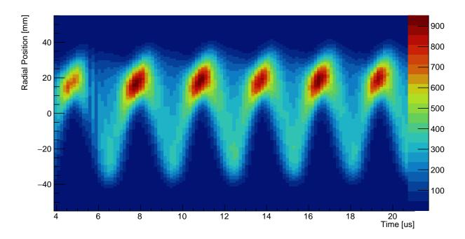
Figure 3.75: Resolution- and acceptance-corrected radial position versus time from tracker data, Station 12. By reconstructing the trajectory of decay positrons detected by the tracking planes, muon decay positions are extrapolated. Coherent oscillations are a consequence of the beam injection process.
