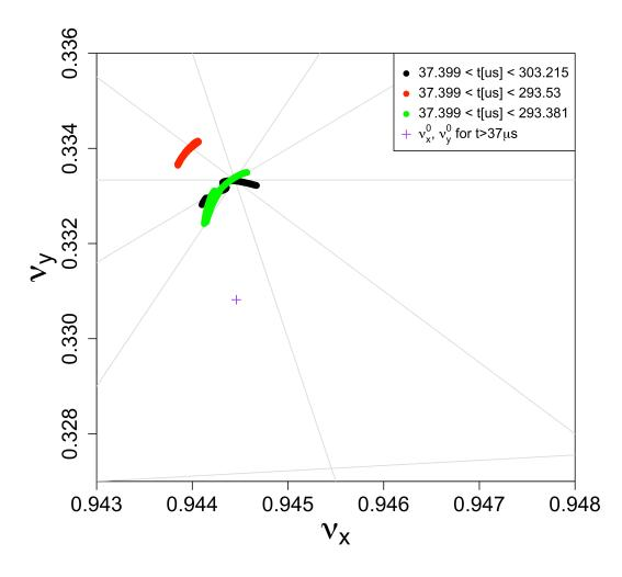
Figure 3.42: Tunes of three muons in the nonlinear regime before getting lost.
