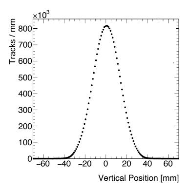
Figure 1.14: Vertical beam profile from the tracking detection system [45].
