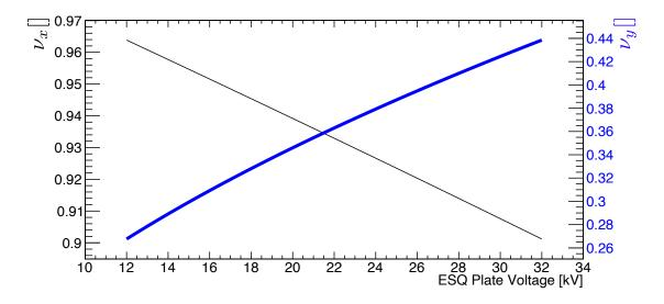
Figure 3.15: Radial (black) and vertical (blue) betatron tunes as a function of ESQ voltage. linear chromaticities  $\xi_{x,y}$ , defined as
