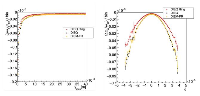
Figure 4.23:  $\langle \Delta \omega_a \rangle$  spread binned over vertical betatron amplitudes (left) and momentum offsets (right) for the case of full betatron motion.
