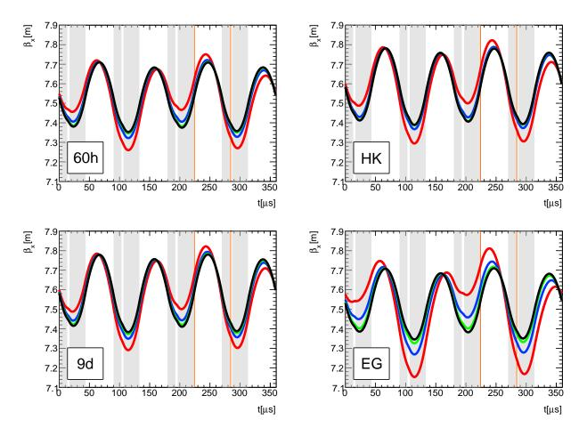
Figure 3.70: Radial beta functions at  $30 \,\mu s$  (red curves),  $100 \,\mu s$  (blue curves),  $200 \,\mu s$  (green curves), and  $300 \,\mu s$  (black curves) during Run-1.
