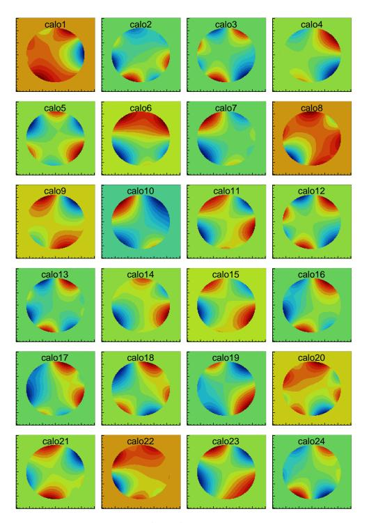
Figure 4.27: Magnetic field maps  $B_i(x_j, y_k)$  from trolley run number 3956 (close to the Run-1a data period). The azimuthal locations of each map correspond to the beam profile azimuths arrangement in Fig. 4.26. Field intensities are shown for  $\sqrt{x^2 + y^2} < 45$  mm, where the horizontal and vertical axes are x and y, respectively. Each color represents a particular magnetic field magnitude to illustrate polar uniformities.
