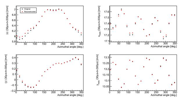
Figure 4.35: Time-integrated beam centroids and widths over the azimuthal angle. Red markers correspond to reconstructed beam profiles  $M_T^{reco}(x, y, \theta_i)$ , whereas entries from the simulated beam profiles  $M_T^{orig}(x, y, \theta_i)$  are shown in black.
