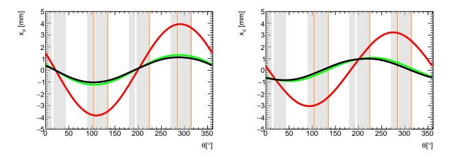
Figure 3.23: Radial closed orbits ( $\delta = 0$ ) at 5 µs (red curves), 20 µs (green curves), and 1000 µs (black curves). On the left-side plot HV = 18.3 kV, whereas HV = 20.4 kV for the plot on the right side. The intentional stretching of the orbit during scraping increases the probability of outermost muons to hit a collimator and, in this way, minimize muon loss rates.
