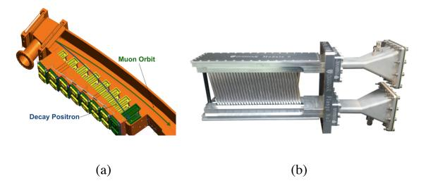
Figure 1.7: (a) Straw tracking station and (b) a detector module [38].
