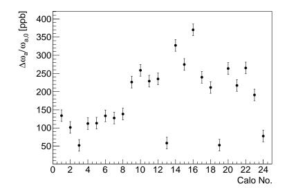
Figure 4.17:  $\omega_a$  shifts induced by phase-acceptance drifts from experimental data (Run-1d) [44]. The Run-1d COSY-based optical lattice functions and per-calorimeter maps from GM2RINGSIM (T-Method) are utilized to calculate all the precession corrections from phase drifts extracted with the randomization method. Courtesy of Elia Bottalico.
