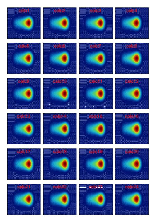
Figure 4.34: Run-1a reconstructed beam transverse profiles  $M_T^{reco}(x_j, y_k, \theta_i)$ , integrated over 30 µs < t < 300 µs. The 24 azimuthal locations coincide with the regions of maximum calorimeter detection acceptance. Horizontal and vertical axes correspond to -60 mm < x < 60 mm and -60 mm < y < 60 mm. Refer to Fig. 4.36 for the color legend.
