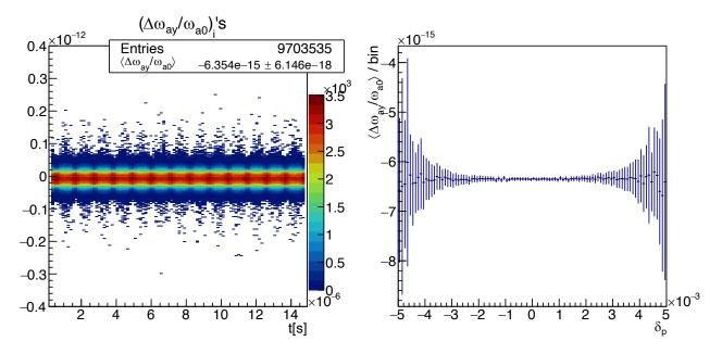
Figure 4.19:  $\langle \Delta \omega_a \rangle$  spread versus time (left) and momentum offset (right). Muons are contained in the horizontal midplane, the magnetic field is uniform and oriented in the vertical direction, and the ESQ is turned off.
