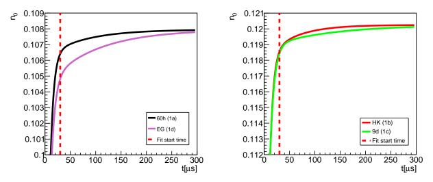
Figure 4.24: Effective field indices over time during Run-1 from straw trackers data  $(n_0 = 1 - \left[1 - \omega_{CBO,x}/2\pi f_c\right]^2)$ .
