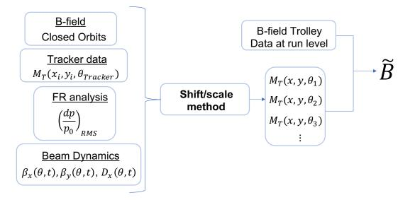
Figure 4.33: Flow chart of the method to reconstruct  $\tilde{B}$  from experimental data and the optical lattice. With this input, beam transverse profiles  $M_T(x, y, \theta_i)$  are methodically prepared in the experiment. Tracker data input on the left of the chart refers to the beam transverse profiles measured by the muon g-2 straw tracking detectors [38].
