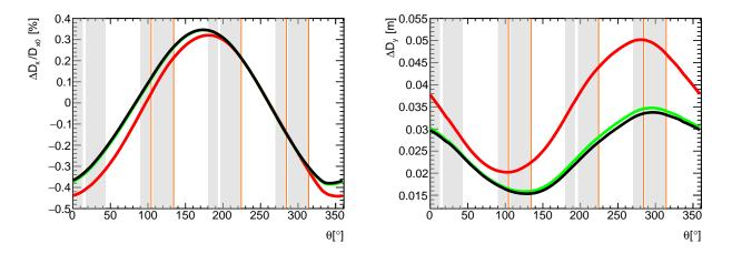
Figure 3.22: Dispersion function distortions from magnetic field inhomogeneities at 5  $\mu$ s (red curves), 20  $\mu$ s (green curves), and 1000  $\mu$ s (black curves) for HV = 18.3 kV. The plot on the right side shows the total distortion in the vertical dispersion function, which is equal to zero in the nominal case, whereas on the left side the relative distortion of the radial dispersion function is displayed.
