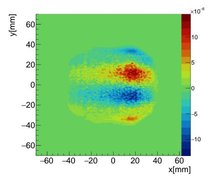
Figure 4.37: Difference between reconstructed  $M_T^{reco}(x, y)$  and original  $M_T^{orig}(x, y)$  beam transverse profiles azimuthally averaged and integrated in time (30 µs < t < 300 µs). Higher order beam moments unaccounted-for in the method to reconstruct profiles  $M_T^{reco}$  introduce discrepancies with the reference case  $M_T^{orig}$ .
