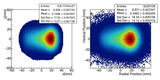
Figure 3.77: Muon beam intensity from simulation (left) and tracker data (right), station 12, during Run-1a from  $30 \,\mu s < t < 300 \,\mu s$ .
