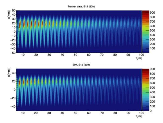
Figure 3.79: Radial beam evolution over time from tracker S12 data (top) and simulated beam (bottom) during Run-1a. The data-driven reconstruction of the initial beam conditions allows to capture in beam tracking simulations (in this case with the COSY-based model) the transverse and temporal evolution of the observed beam.
