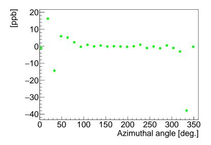
Figure 4.38: Relative differences between reconstructed and original muon-weighted fields  $(\tilde{B}_{i,reco} - \tilde{B}_{i,orig})/\tilde{B}_{i,orig}$  over the azimuthal angle. Largest discrepancies emerge at azimuthal regions where the field is less uniform (i.e., at 335° and 25° around the inflector and magnet leads, respectively).
