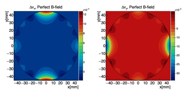
Figure 3.26: Amplitude-dependent tune shifts ( $\delta = 0$ ) within the storage region without magnetic field imperfections (HV= 18.3 kV). The horizontal axis corresponds to radial betatron amplitudes and the vertical axis represents vertical amplitudes.
