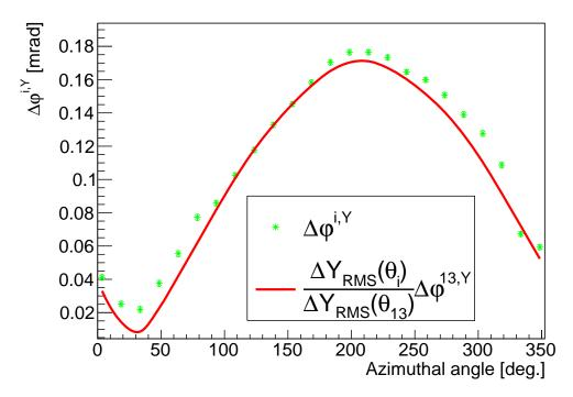
Figure 4.12: Drifting phase amplitudes from single-exponential fits to phase drifts (extracted from non-randomized, sliding window fits) induced by vertical beam motion. In red, scaling of the phase amplitude at calorimeter k = 3 with vertical beam width drifts only.
