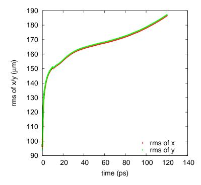
Figure 5.19: The transverse bunch sizes evolve with time
