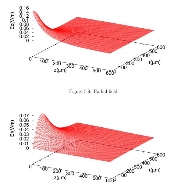
The longitudinal field and the radial field on the grid of one unit charge with Gaussian distribution on the surface are shown respectively in Figure 5.8 and Figure 5.9. We assume the charge distribution of the positive residuals does not charge, only the number of charges changes and it is always equal to the number of electrons outside the surface. So at any time,
