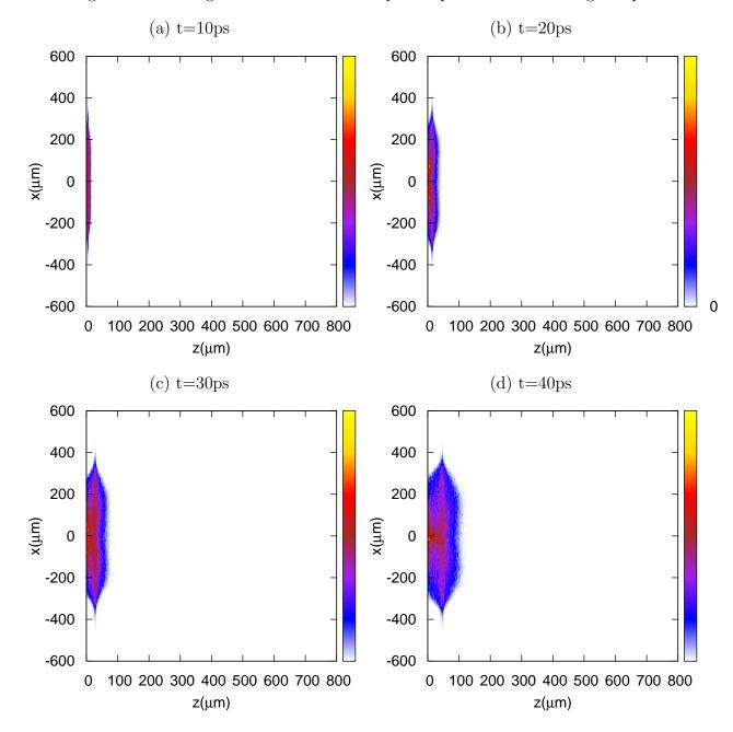
Figure 5.22: Charge distribution in x - z phase space in the following 120 ps
