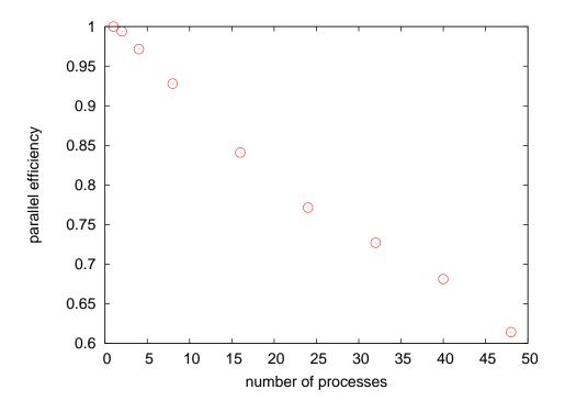
Figure 4.13: Parallel efficiency for 1,000,000 electrons with different number of processes
