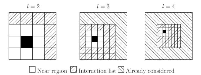
Figure 2.3: The behavior of the interaction list of boxes at three levels
