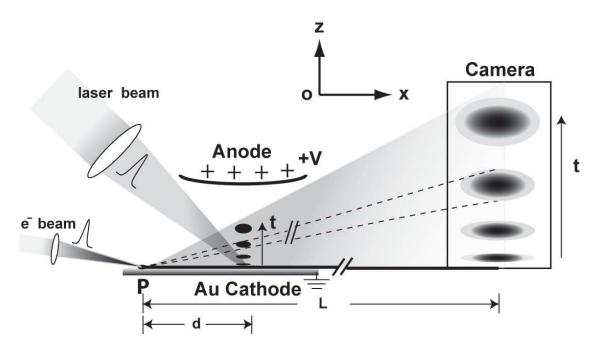
CCD camera. The position and the size of the bunch can be obtained by measuring the shadow patterns and fitting the experimental data with an analytical expression describing the projection geometry [75].
