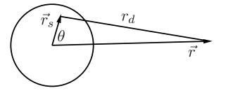
In order to give an error estimation of the far multipole expansion of the charges, let us first consider a source charge inside a spherical region of radius a as shown in Figure 3.1.
