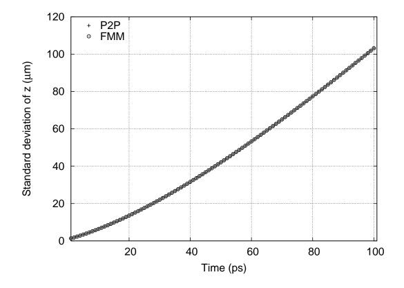
Figure 2.9: Longitudinal bunch size during the free expansion of an electron bunch
