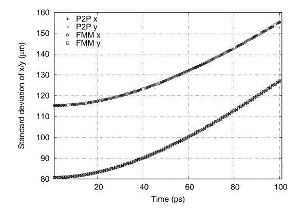
Figure 2.10: Transverse bunch size during the free expansion of an electron bunch
