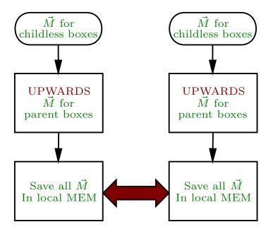
Figure 4.9: Parallel multipole expansion calculation
