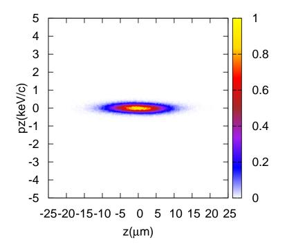
Figure 5.4: Electron density in  $z - p_z$  phase space
